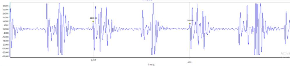
Figure 1 Time Signal clearly shows peaks within 0.0167 seconds which indicates 60 Hz
