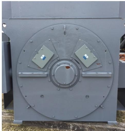
In addition, CAP-ENV-24 windows were mounted on the main incoming cable termination chamber of the motor skid to allow inspection of the main cable terminations and the large Medium Voltage starter capacitor terminals.
