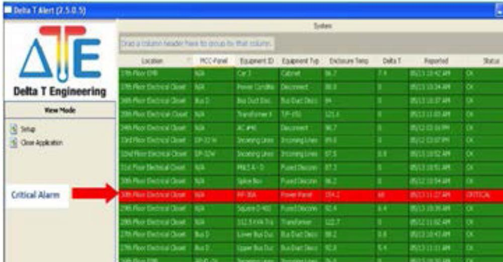
Figure 1 30th Floor Electrical Closet Panel RP-30A shows an operating status as “Critical” with a Delta T of 68°F.
